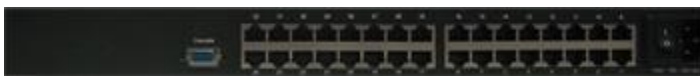
Close up of the Rear View of Cat-6 KVM showing Qty 16 RJ45 interface Ports
